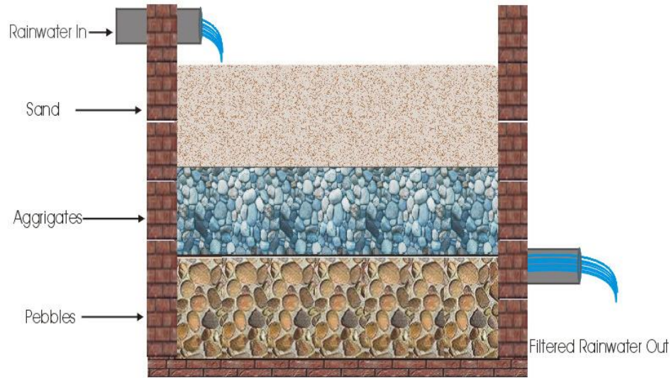
Figure 7 Design of Rainwater harvesting pit
